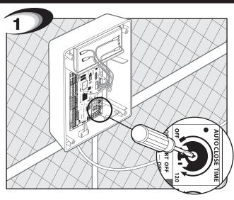
Turn the "AUTO CLOSE TIME" arrow in the center of the potentiometer with small flat head screwdriver. Turning the pot all the way counter-clockwise will turn the auto close feature off. The minimum auto close time is 3 seconds. The maximum (turn the pot all the way clockwise) auto close time is 120 seconds.
