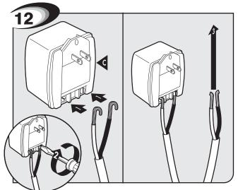
Cut excess cable/strip 1/2" off 2 wires/twist ends. Attach wires to transformer screw terminals. NOTE: The Mighty Mule power input is not polarized. The wires can be inserted into either terminal regardless of color.
