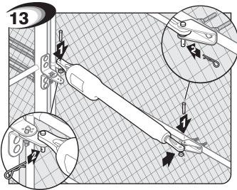
Attach and secure opener assembly to brackets.
