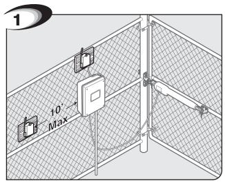
Install Receiver within 10 ft of control box (longer lengths available - call us). NOTE: NEVER splice receiver cable. DO NOT run cable through metal conduit because the receiver signal range will decrease. DO NOT run cable through conduit containing AC wire. DO NOT place receiver within 3 feet of AC
