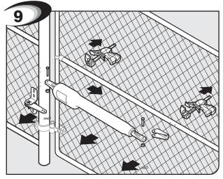
Remove clamps, post, gate brackets, and opener. Then use a hammer and center punch to dimple the hole positions for drilling.
