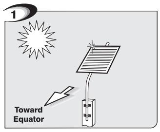
The solar panel must be positioned facing the path of the sun and in an open area away from shade. It should receive at least 8 hours of direct sunlight for a full charge.
