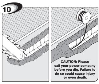
Dig trench and lay wire from AC power source to control box. Use only 16 gauge multi-stranded, low voltage, PVC sheathed wire (RB509). NOTE: DO NOT use telephone wire or solid core wire. NEVER splice wires together. We recommend running wire in PVC conduit.
