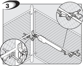
With Gate in OPEN position, using clamps, secure opener to gate post and center cross member of gate.
