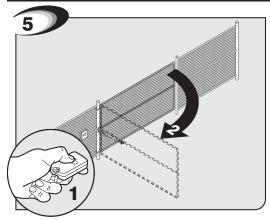
Press button on opener remote to open gate.
