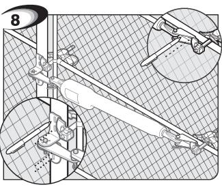
Mark middle of post bracket slots on fence post. Mark middle of gate bracket slots on gate cross support.
