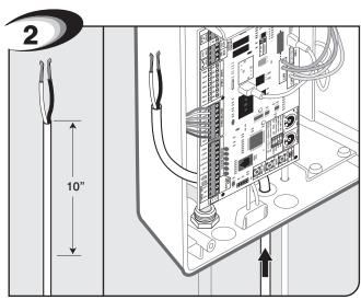
Feed 10" of wire from solar panel into box through the predrilled hole in the bottom of the control box.
