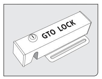
For use exclusively with GTO Lock (FM143 or FM144). Connecting other devices to these terminals may cause incorrect operation and void your warranty. You do not use the lock board with this control board.
