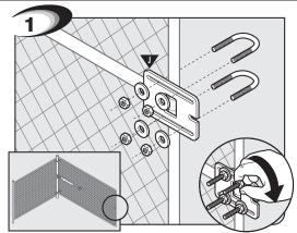
Fully open gate. On push-to-open gates attach gate stop on the outside of the gate with one of the following:
