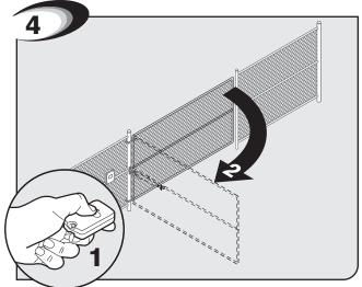
Press button on opener remote to fully open gate. Closed limit is set upon reaching fully open position. Test and, if needed, reset and start over.
