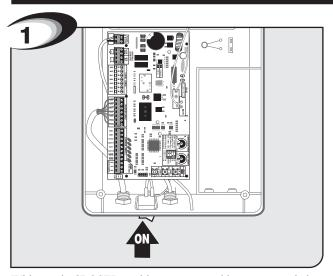
With gate in CLOSED position, turn control box power switch
