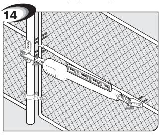
Check for level. Adjust post bracket if necessary.
