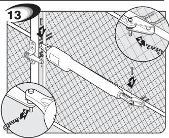
Attach and secure opener assembly to brackets.
