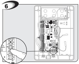
Hold the "LEARN MASTER LIMIT" button for 10 seconds, or until the alarm sounds to clear. Go back to setting open gate limit step 1 at the top of this page.
