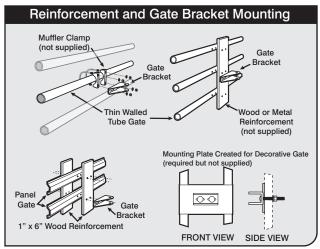
Recommended reinforcement and gate bracket mounting
