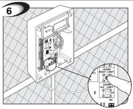
Press and hold the "LEARN MAST LIMIT" button for 10 seconds, or until the alarm sounds to clear. Go back to the setting closed limit steps on the top of this page.
