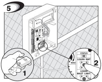
Release the remote button, then release the "LEARN RMT" button. The new code is now programmed. Fill in boxes below with your transmiter code for your records.
