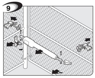
Remove clamps, post, gate brackets, and opener. Then use a hammer and center punch to dimple hole positions for drilling.
