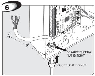
Feed cable 6" through the strain relief bushing into control box. Tighten strain relief bushing nut and secure cable by tightening the sealing nut.
