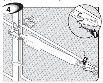
Remove clevis pin from the gate bracket and support loose opener.
