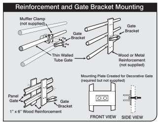
Recommended reinforcement and gate bracket mounting examples (muffler clamp does not require drilling and is adjustable).
