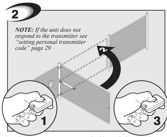
Press button on opener remote; gate should start closing. Press button on opener remote again when gate is in desired CLOSED position. **NOTE:** if the gate stops and reverses see "setting obstruction stall force" page 28.
