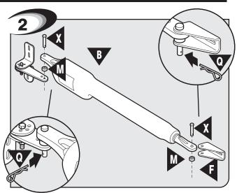
Attach opener to gate bracket and secure with hardware required.
