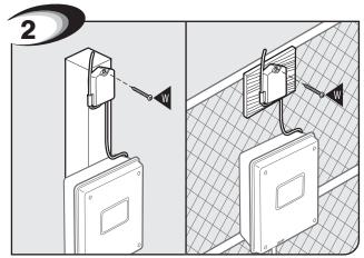
Check Receiver/Remote signal reception in mounted position/OK secure Receiver in position to fence or post. NOTE: If mounting on metal fence, mount receiver on a piece of wood. Mounting the receiver on metal can cause interference and the receiver may not work properly. DO NOT mount upside down.
