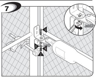
Secure post pivot bracket to post bracket when clearances are OK (Step 5) in both open and closed positions.
