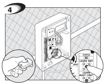
Go to control box. Press and hold the remote and "LEARN RMT" buttons simultaneously for 5 seconds or until the alarm sounds.
