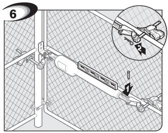
OPEN gate and re-attach opener with clevis pin. Check for level. Clamp securely.
