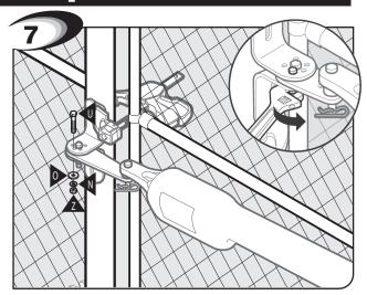
Secure post pivot bracket to post bracket when clearance is OK (Step 5) in both open and closed positions.
