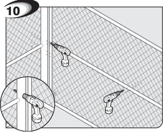
Drill 3/8" holes completely through gate post and gate cross support.
