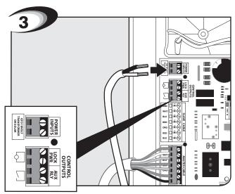
Insert wires from the solar panel into the 18V Power Input terminal. The 18V Power Input terminals are not polarized, so the wires can be connected regardless of polarity or color.
