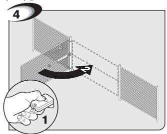
Press button on opener remote to fully close gate. Open limit is set upon reaching the fully closed limit. Test and, if needed reset and start over.
