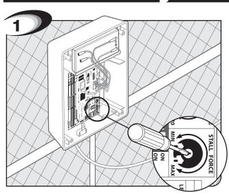
Do not use the Dual Sense Stall Force adjustment to compensate for a gate that is sticking or binding. Excessive Stall Force may cause damage to the gate operator or gate system or Injury or Death.
