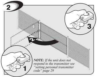
Press button on opener remote; gate should start opening. Press button on opener remote again when gate is in desired OPEN position. **NOTE:** if the gate stops and reverses see "setting obstruction stall force" page 28.
