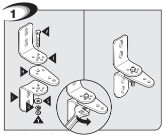
Assemble post bracket parts.
