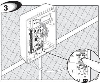
Press and hold the "LEARN MAST LIMIT" button for 5 seconds, or until the alarm sounds.
